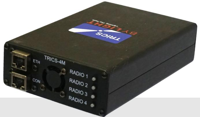
The Tactical Radio Over Internet Protocol (RoIP) Inter-Communications System (TRICS) is a radio gateway network appliance that enables IP access to radios.
