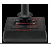
If the Throttle is pulled back during start, the vehicle will begin the experience driving in reverse.
